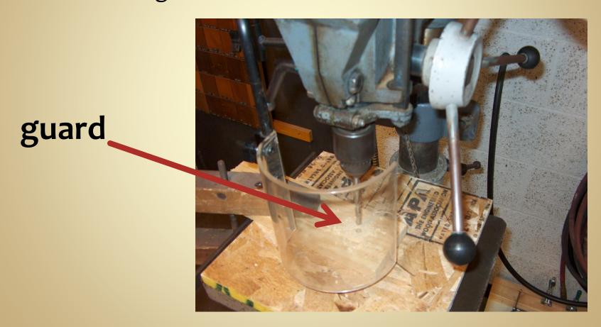
Only set the depth stop when the machine is stopped
