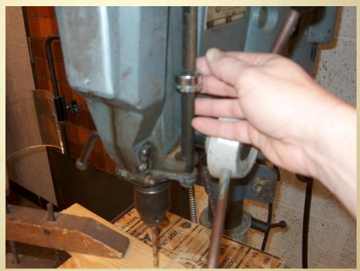
Never try to stop a piece of wood that is spinning on the drill press
