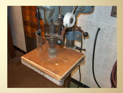
Make sure the bit is in the chuck straight and tighten it securely with the chuck key
